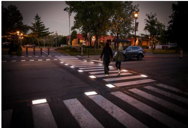
Fig. 1 Newly installed lighting system in Candia, Quebec, Canada, for improving intersection traffic safety. The image is adopted with permission from the Ville de Candiac [Source].
